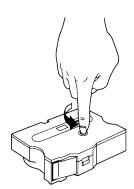
6. Insert the tape cassette firmly into the cassette compartment.
