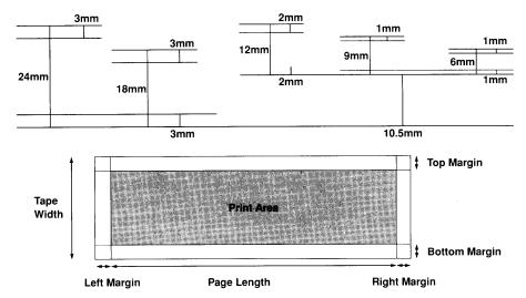
The page maximum length is 1 m regardless of the tape width. Left and right margins are as follows:
