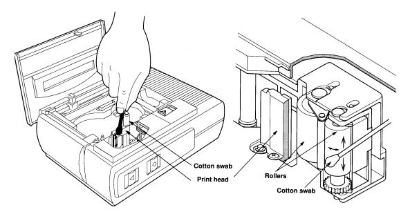
**Warning:** Do not touch the printer head with your finger. The printer head becomes hot when working, and remains hot for a while after the power has been switched off.
