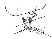
You can use reverse sewing for locking the end of seams and where you need to strengthen a stitch.
