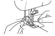
Hold the thread in front of the needle to make sure that the hook grabs it.
