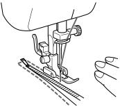
To sew the opposite side of the zipper, release the foot by raising the lever located at the back of the presser foot, position the zipper foot on the other side of the zipper and continue sewing using the notch on the other side.
