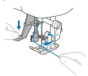
► The end of the needle threader rotates toward you and the hook passes through the eye of the needle.
