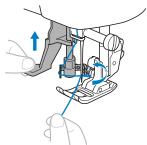
Pull out about 5 cm (2 inch) of thread through the needle toward the back of the sewing machine.
