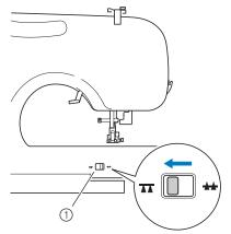
① Feed dog position lever (as seen from the rear of the machine)
