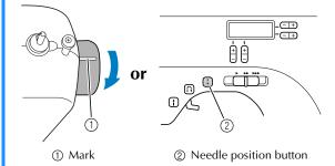
If the needle is not correctly raised, the sewing machine can not be threaded. Be sure to turn the handwheel so that the mark on the wheel points up before threading the sewing machine.
