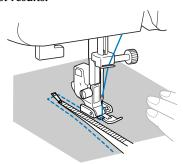
To sew the opposite side of the zipper, release the foot by pressing the button located at the back of the presser foot, fit the zipper foot on the other side of the zipper and continue sewing using the other side notch.
