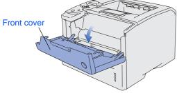
Unpack the drum unit assembly. Rock it from side to side several times to distribute the toner evenly inside the assembly.
