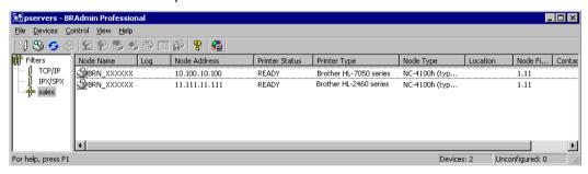
The BRAdmin application can use the IPX/SPX or TCP/IP protocols to communicate with the Brother print server. As the default IP address of Brother print servers is 192.0.0.192, the print server will probably be incompatible with the IP address numbering scheme on your network. If you are not using DHCP, BOOTP or RARP, you will want to change the IP address. There are two ways that you can do this from within BRAdmin.
