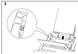
Load paper into the multi-purpose sheet feeder.
