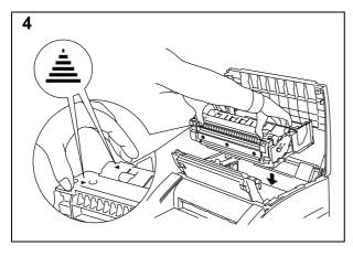
Install the drum unit into the printer.
