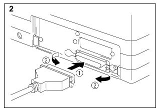
Connect the parallel interface cable to the parallel interface port of the printer. ( 1 )
