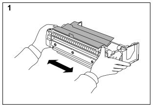
Unpack the drum unit and gently shake it from side to side five or six times.
