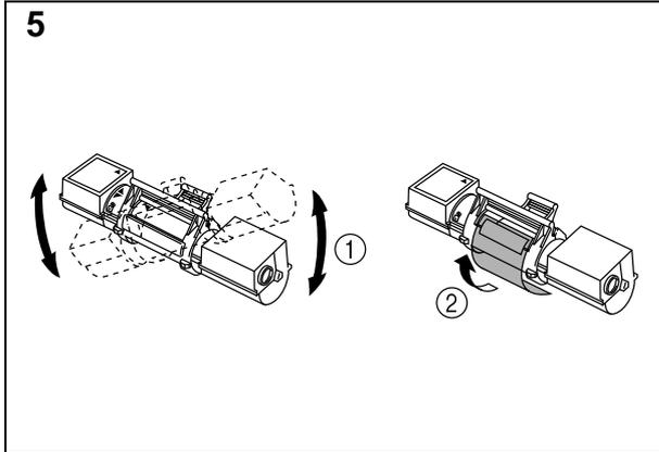
Unpack the toner cartridge and gently rock it from side to side well before installing.
