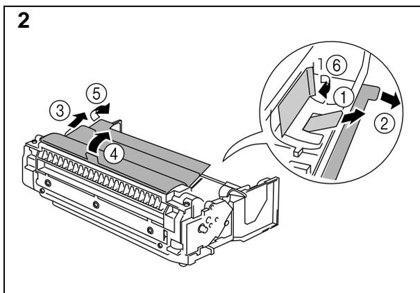
Remove the protective parts, in order, as shown in the illustration.
