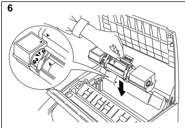
Install the toner cartridge into the drum unit. Make sure that the ▲ marks are aligned.
