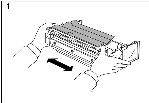
Unpack the drum unit and gently shake it from side to side five or six times.
