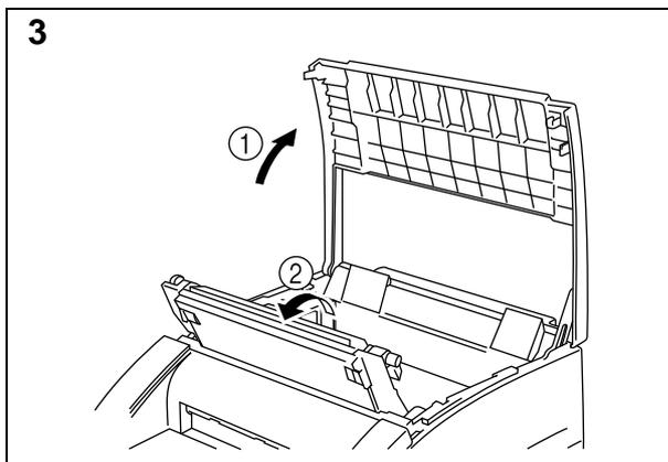
Open the top cover. Open the drum cover by pushing the two blue tabs in toward the center of the unit and lifting the cover toward you.
