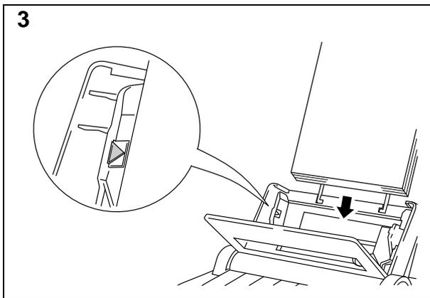
Load paper into the multi-purpose sheet feeder.
