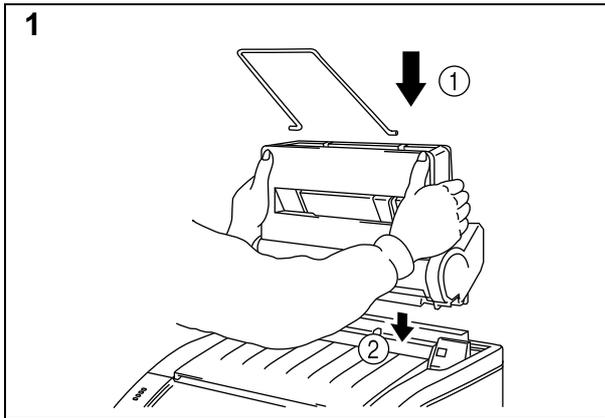
Install the paper support into the multi-purpose sheet feeder. (①)
