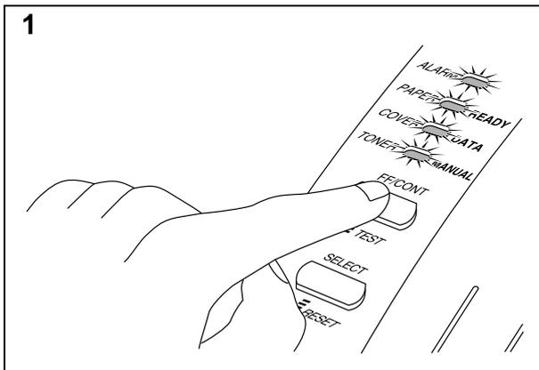
Depress the TEST (FF/CONT) switch until all lamps are turned ON. The printer starts printing a test sample page.
