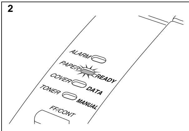
Make sure that the READY lamp is ON after the printer has warmed up (about 60 seconds).
