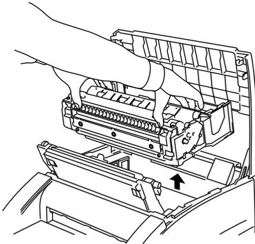
**2 Place it in the plastic bag and fold the plastic bag under the drum unit.**
