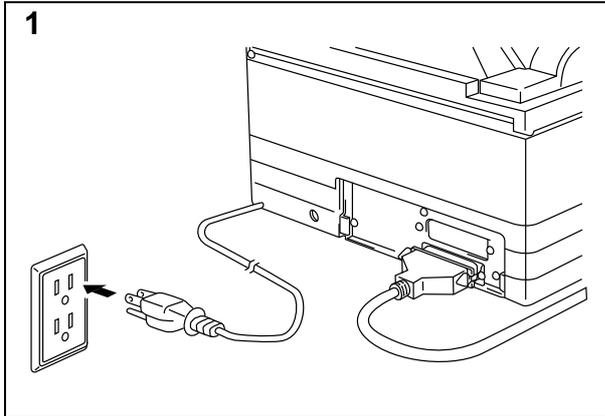
Plug the power cord into the AC power outlet.
