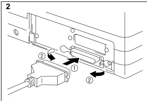
Connect the parallel interface cable to the parallel interface port of the printer. ( ① )
