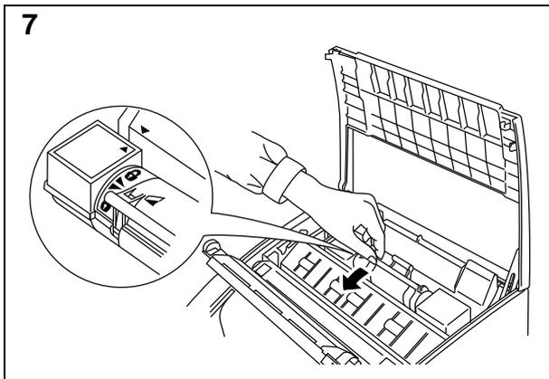
Gently pull the blue shutter lever on the toner cartridge forward until the red arrows are aligned.
