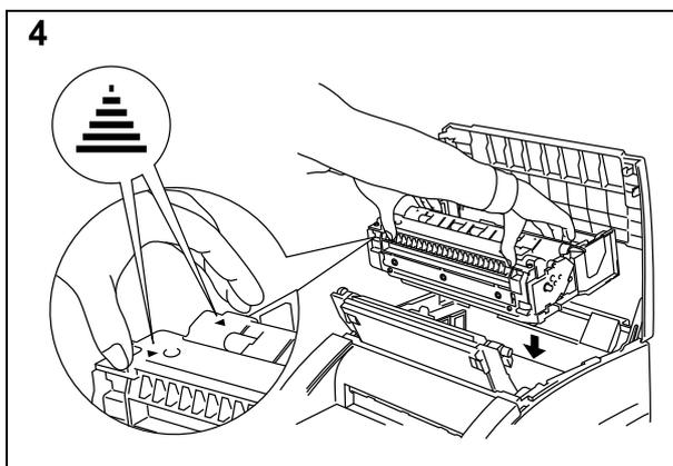
Install the drum unit into the printer.
