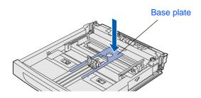
5 Squeeze the length guide and slide it to fit the paper size.
