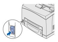
2 Hold down the button as you turn on the power switch. Keep the button pressed down until the LCD display shows READY.
