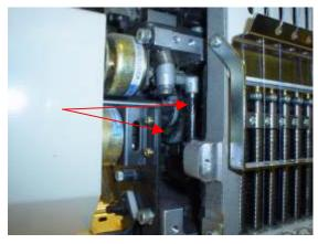
8. Reinstall arm covers if supplied. Manually color change the machine to needle 1 by rotating the knob underneath the color change box. Remove the presser foot guides by removing the 3 screws.
