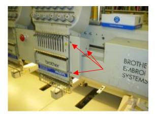
4. Remove the cover to the left on head 6 by removing the 3 screws.
