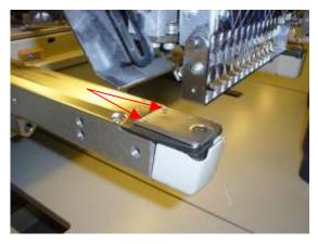
Clean any thread and lint around the moving and fixed knives with a brush or compressed air. Do this for all heads.
