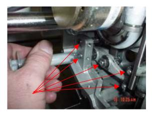
18. Remove the one screw on the left of the head and inject grease into the hole. Replace screw.
