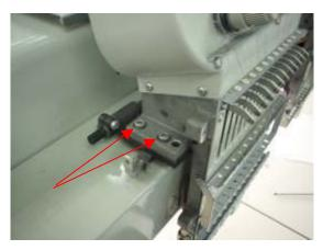
10. Cut threads between thread stand and head. Remove head from machine by lifting up on it and unhook the wire clamp and disconnect the 2 connectors at the back. Do this for all heads.
