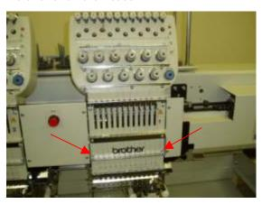
2. Oil each needle bar as shown in the picture by placing a small drop of oil on each needle bar in the two locations. Do this for all the needle bars on all the heads.
