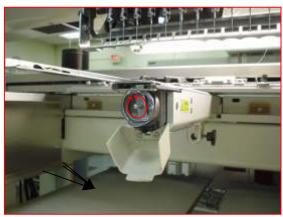
2. Insert bobbin cases in to rotary hooks. Make sure bobbin thread is not over 2 inches long. Close bobbin case covers.
