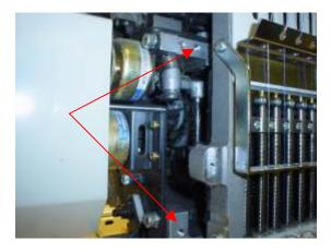
15. Remove the presser foot guide plates by removing the 3 screws and unhooking the spring from the rear of the plates.
