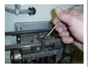
20. Apply black grease to the presser bar spring, end of presser bar guide bracket, presser shaft bushing and jump rotary shaft as indicated by arrows.
