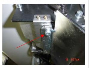
12. Loosen this bolt and let the cap eaves guide hang down.
