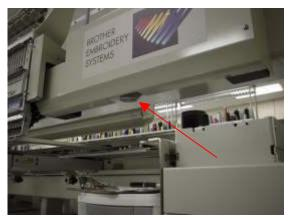
6. Remove the arm cover on the heads if the machine has them by removing the 2 screws. *Cover is not shown in photo.*
