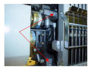
7. Using the black grease, grease the groove of the thread take up cam. Wipe a little grease on the base needle bar. Do this for all the heads.
