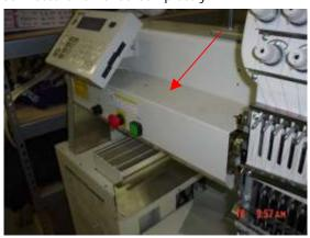
6. Remove the color change assembly cover by removing the two top screws and loosening the 2 bottom screws.
