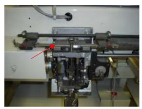
22. Grease the V groove both sides of the linear rail for the color change assembly with white grease. Grease the color change assembly and roller bearings with black grease.
