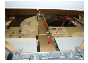
4. Using the white grease, lubricate all of the linear rails in the V groove both sides of the rails for X-axis, Y-axis plus the linear rail inside the sewing arm of head 3. You will have to move the pantograph both front to back and left to right to lubricate all the grooves.
