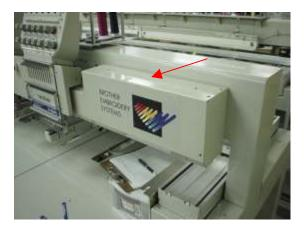
7. On 4 head models. Remove the color change rod cover by removing the 2 screws.
