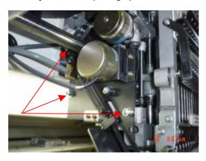
14. Remove the left arm cover on the heads if the machine has them by removing the 2 screws. *Cover is not shown in photo.*
