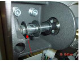
24. Grease the wiper assembly slot top and bottom with white grease on both left and right sides.
