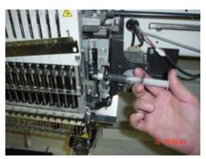
19. Remove setscrew at top of base needle bar and inject grease in to hole. Replace setscrew.
