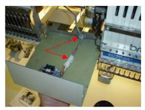
3. Remove the cover to the right of head 1 by removing the 3 screws.
