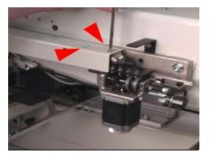
8. Manually color change the machine in between needles 4 and 5 on 9 needle machines or between 6 and 7 on 12 needle machines by rotating the knob underneath the color change box.
