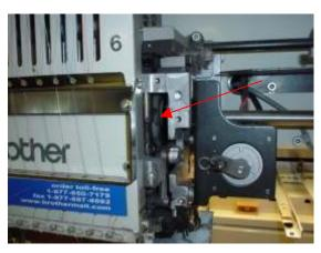
11. Hook the spring to the back of the presser foot guide plate and reinstall the plate leaving the screws loose. Make sure that the shaft clamp of the presser foot goes into the guide on the plate. The retracting lever should be underneath the shaft clamp. Before final tightening of the screws, please check the alignment of the presser foot to the needle plate and make sure that the presser foot goes up and down smoothly. Do this for all of the heads.
