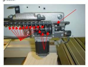
23. Using the black grease, grease the driving shaft thrust bear with black grease by loosening the 2 setscrews on the collar and sliding to the right. Apply the grease to the rollers of the thrust bearing on both sides. Move collar back to the left against the thrust bearing and washer and retighen setscrews. Make sure setscrews ride on the flats of the driving shaft.
