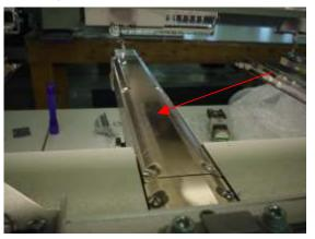
2. Clean the inside of the sewing arm and hook module cooling fan with a brush or compressed air.
