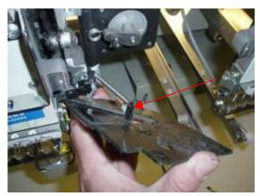
10. Using the black grease, grease the work clamp cam for each head.
