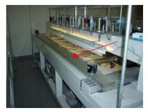
2. Remove the Y-axis covers from each end of the machine by removing the 4 screws for each cover.
