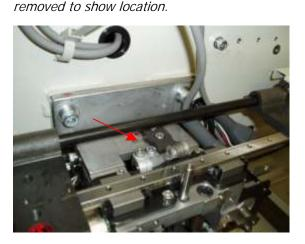
2. Place 1-2 drops on the thread take up bushing on each head. *Head has been removed to show location.*
