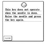
This message is displayed when a button on the screen is pressed while the needle is lowered.
