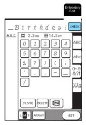
Press ARRAY to change the layout of the pattern.
