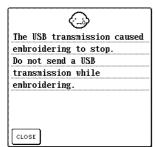
If data is being written to or deleted from "Removable Disk" on the connected computer during sewing, the machine stops and this message is displayed. When the USB transmission is completed, press the "Start/Stop" button to continue sewing.
