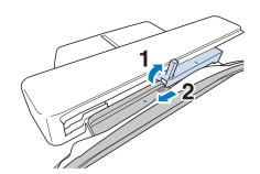
Insert a wound bobbin into the machine. (see "Setting the Bobbin" of "Basic operations".)
