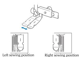
Change the needle position so that the needle does not touch the presser foot.
