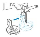
Tighten the screw with the included screwdriver.
