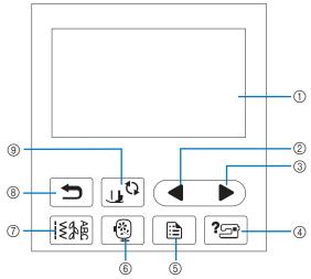
1) LCD (liquid crystal display) (touch panel)
