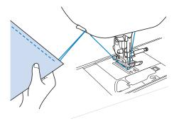
When the needle has stopped moving, raise the presser foot and remove the fabric.
