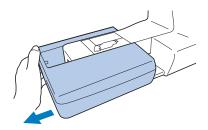
Slide the tab on the cover of the connection port in the direction of the arrow to open the cover.
