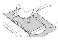
Trim the excess thread at the end of the seam. If the end of the seam is under the presser foot, raise the presser foot, then trim the excess thread.
