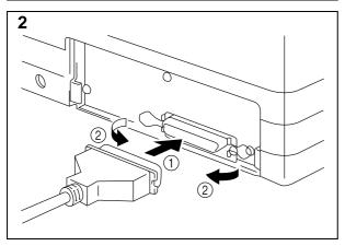
Connect the parallel interface cable to the connector of the printer. ( 1 ) Secure the connection with the wire clips. ( 2 )
