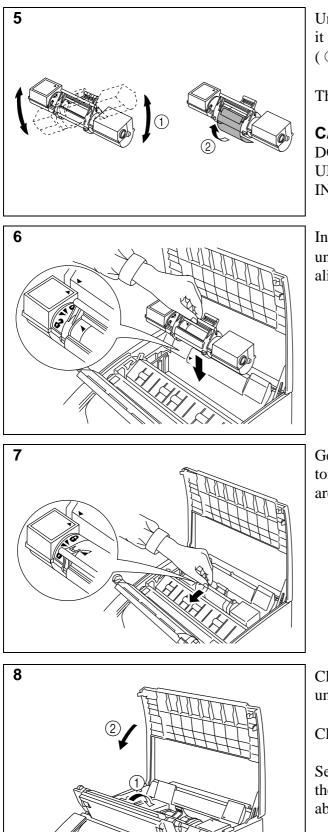
Unpack the toner cartridge and gently rock it from side to side well before installing. (1)
