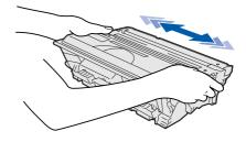
4 Put the drum unit assembly into the printer.
