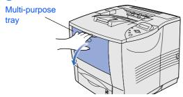
3 Remove the protective part from in the multi-purpose tray.
