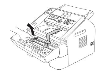
• Pull the paper strip to remove the protective material as shown in the illustration.
