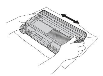
**h** Put the drum unit and toner cartridge assembly back in the machine.
