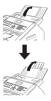
• Open the control panel cover by lifting it toward the back.
