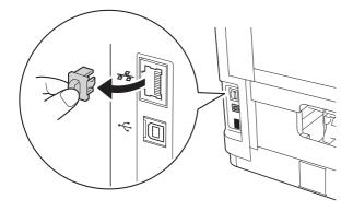
C Connect the network interface cable to the Ethernet port, and then connect it to a free port on your hub.
