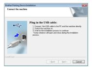
Connect the USB cable to the USB port marked with the e symbol on your machine, and then connect the cable to your computer.
