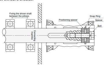
Figure-4 Fixing by spacer and snap ring
