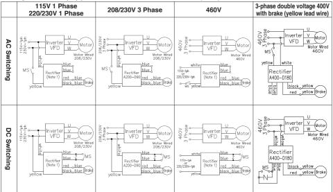
Note 1: If the input power is 115V 1 phase, use Rectifier A100-D90. If the input power is 220/230V, use Rectifier A200-D90. (Input power to the brake is 90vdc)
