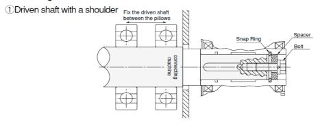
Figure-2 Fixing by spacer and snap ring
