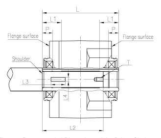
Figure-6 Recommended Dimensions of the Driven Shaft
