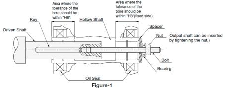
(Spacer, nut, bolt, key and jig parts are not supplied by Brother)
