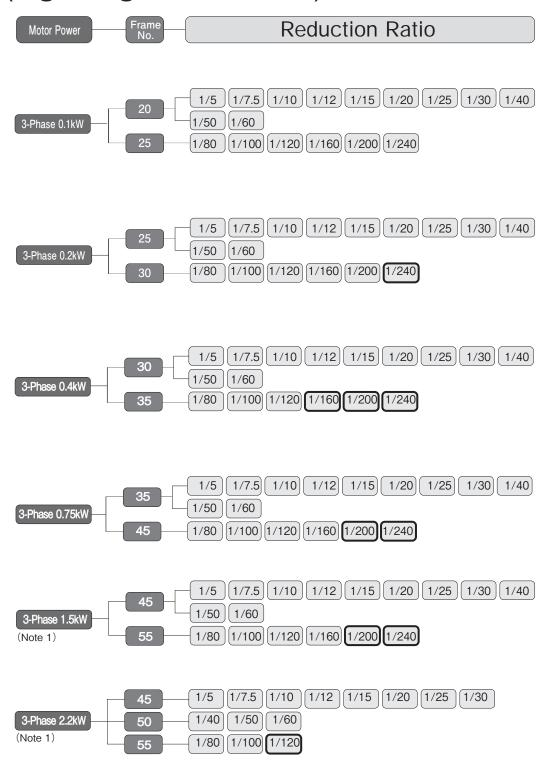
(Notes) 1.1.5kW and 2.2kW IP65 models cannot be provided with a brake.
