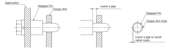
Figure 7: Example of Stepped Pin Usage
