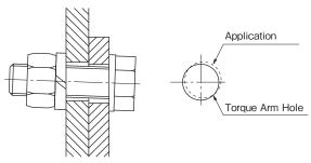
Unnecessary force applied to the drive shaft and hollow bore can result in defects.
