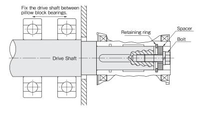
Figure-2: Attachment Using a Spacer and Retaining Ring (Customers need to provide their own spacers, bolts, and retaining rings)
