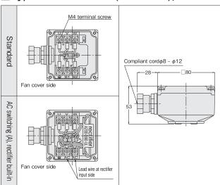
(Note) 1. When a brake motor is attached, the brake lead wires are taken out loosely form the brake unit.
