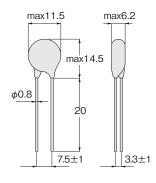
Appropriate for cutting off the sparks of a brake switch for AC line switching.
