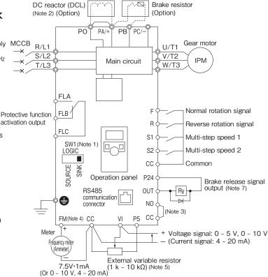
■Example of connections at the source (Common: P24) side
