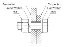
Figure 6: Fastening the Detent
