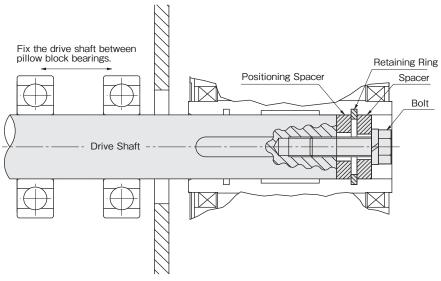
Figure-4: Attachment Using a Space and Retaining Ring
