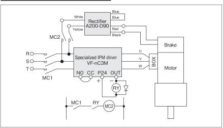
(Note) 1. The function of output terminal OUT utilizes the "Brake open signal" (Function No. 68 [Positive logic], 69 [Negative logic]). (Function No. 68 has already been assigned when shipped from the factory.)
