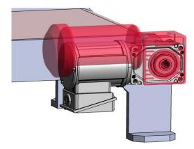
Figure 8: Worm vs. Hypoid Gearmotor Footprint Comparison
