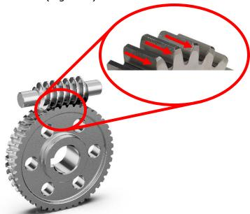
**Figure 2: Sliding Friction Visualization**
