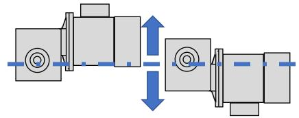
Figure 9: Worm vs. Hypoid Gearmotor Shape Comparison
