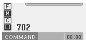
3. Input the zigzag stitch length in 3 digits, and then press **M**.
