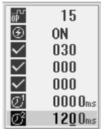
3. Referring to the table of condition numbers of the extended option output (see page xxx), set the output condition for No. 16 to "condition No. 98 (when No. 15 is turned on)". Set Timer 1 to 0.5 sec. (500 ms) and Timer 2 to 0.7 sec. (700 ms). On the setting screen, make the following settings.
