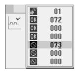
3. Referring to the table of external input condition numbers (see page 151), set "ON when condition No. 40 (input 1 ON) is established" as the output condition for No. 2 ON. On the setting screen, make the following settings.
