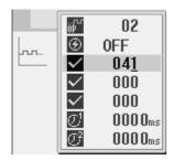
5. Referring to the table of external input condition numbers (see page 151), set "enabling when condition No. 42 (input 1 ON) is established" as the enabling condition for No. 2. Set "disabling when condition No. 43 (input 2 OFF) is established".
