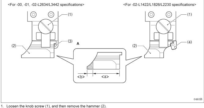
2. [If grinding the hammer (Refer to Figure A)]
