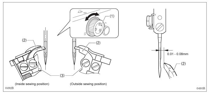
Turn the upper shaft pulley (1) so that the tips of both the left and right loopers (2) are aligned with the needle center, and then loosen the set screws (3) and adjust the clearances between the needle and the tips of the loopers (2) to 0.01 - 0.08 mm.
