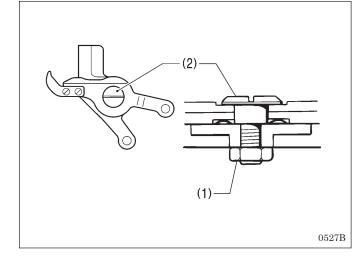
1. Remove the two screws (1), and then remove work clamp plate U (2).
