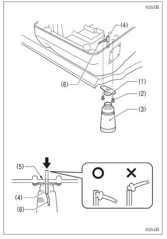
The oiler should be installed while the machine head is tilted back.
