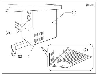
Use a vacuum cleaner to clean the filters in the air inlet ports (2) of the control box (1).
