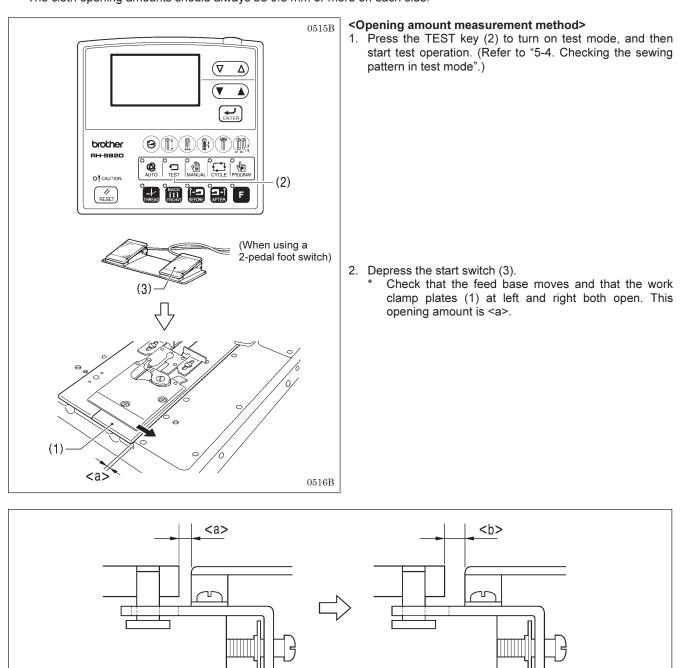
3. Use calipers to measure  $\langle a \rangle$  (at both left and right).
