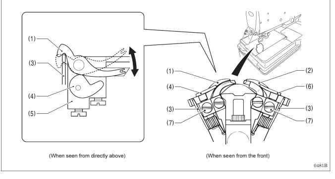
1. Remove the work clamp plates. (Refer to "3-19. Installing and removing the work clamp plates".)
