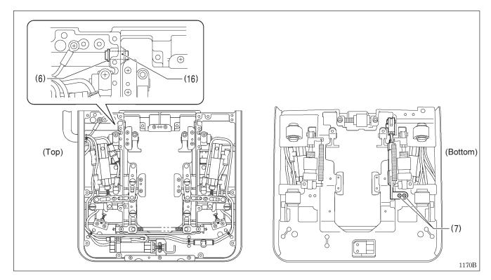
10. Insert the shaft (16) of the auxiliary clamp connecting rod into the hole in the feed base, and then install retaining ring C (6). 11. Tighten the two screws (7).
