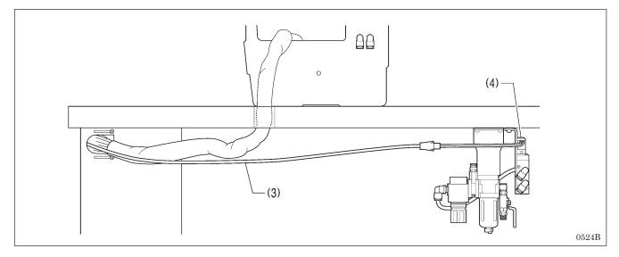
4. Pass the hammer valve harness (3) into the control box through the hole in the rear of the control box.
