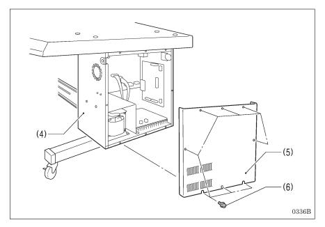
Secure the cover (5) of the control box (4) by tightening the eight screws (6). Check that the cords are not clamped by the cover at this time.
