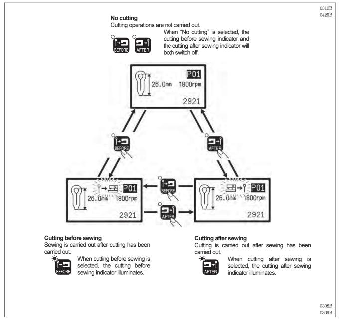
Press the BEFORE or AFTER key during the standby condition in automatic mode, test mode or manual mode. The cutting operation changes as shown in the illustration each time a key is pressed.
