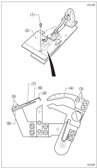
1. Remove the two screws (1), and then remove work clamp plate U (2).
