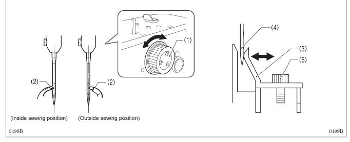
Turn the upper shaft pulley (1) so that the tips of both the left and right loopers (2) are aligned with the needle center, and then loosen the screw (5) and adjust the needle guard (3) so that it touches the needle (4).
