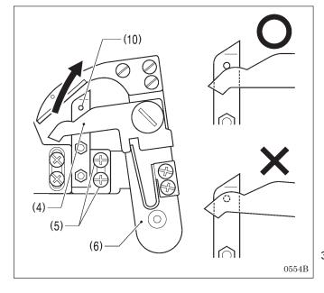
The lower thread must go over the projection (9) on thread nipper M (8) and be held securely. To make sure this happens, check that the operations in (a), (b) and (c) below are all correct.
