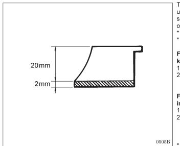
The cutting pressure over the whole of the hammer should be uniform so that the material will be cut cleanly. File the cutting surface of the hammer so that the knife incision will be uniform over the whole of the hammer.
