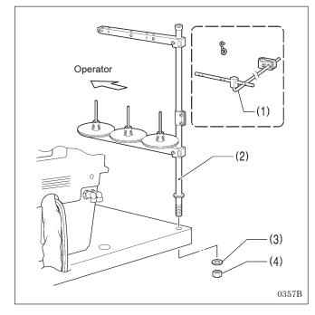
Install the cotton stand so that it is at the far left of the table when looking from the front of the sewing machine.
