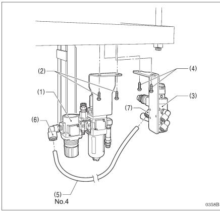
Install to the underside of the table. (Refer to "3-1. Table processing diagram" for the installation positions.)
