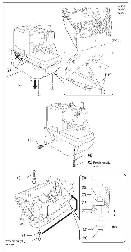
Check that the four bed base cushions (1) have all been installed to the bottom of the bed base, and then place the machine head onto the table.
