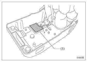
1. When the oiler (1) has filled with oil, turn the oiler (1) to
