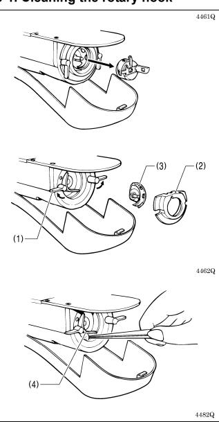
Pull the shuttle race cover downward to open it, and then remove the bobbin case.
