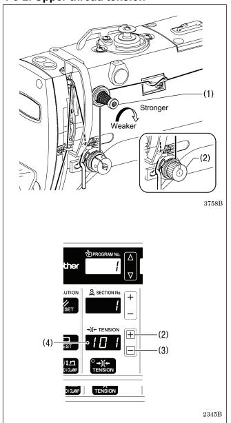
Use the digital tension or the tension nut (2) to adjust the tension as appropriate for the material being sewn. (Refer to "Setting the tension value".)
