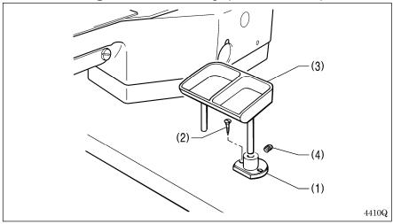
Install the button tray at a place convenient for operation.
