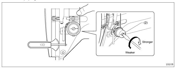
Adjust by turning the shaft (2) with a screwdriver.
