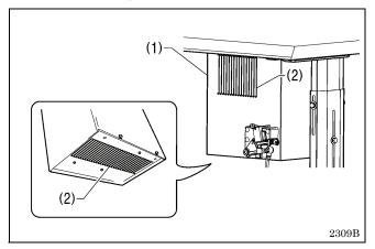
Use a vacuum cleaner to clean the filters in the air inlet ports (2) of the control box (1) at least once a month.
