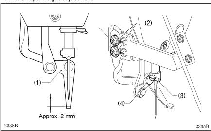
Loosen the two screws (2) and adjust the thread wiper (1) so that the clearance between the top of the thread wiper (1) and the needle point is approximately 2 mm when the thread wiper (1) is aligned with the center of the needle.
