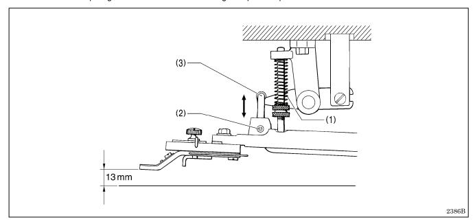
Remove the spring (1), loosen the set screw (2) and adjust the button clamp holder hook (3) by moving it up and down.
