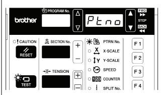
While pressing the TEST key, press the SELECT key.
