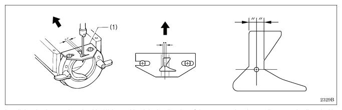
Install the shuttle race thread guide (1) by pushing it in the direction of the arrow so that the needle groove is aligned with the center of the needle plate hole.
