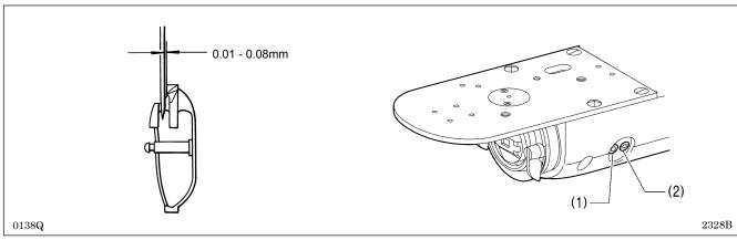
Turn the pulley to align the tip of the rotary hook with the needle center line. Then loosen the set screw (1) and turn the eccentric shaft (2) to adjust so that the clearance between the needle and the rotary hook is 0.01 - 0.08 mm.
