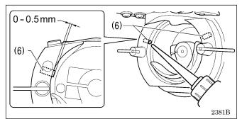
7. Pour oil in through the two holes of the shuttle race base assembly so that the felt (6) is lightly moistened.
