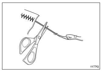
If the upper thread trailing length is 40 mm or more, or if the upper thread tension is weak and the upper thread does not form a good seam at the first stitch, the end of the thread that is being held by the thread nipper may become wound around the seam.
