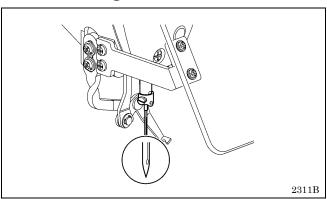
Always check that the tip of the needle is not broken and also the needle is not bent before starting sewing.
