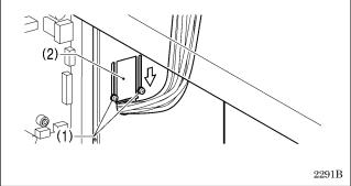
5. Close the cord presser plate (2) in the direction of the white arrow, and secure it by tightening the two screws (1).
