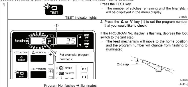
Set the button. (Refer to "4-7. Inserting the button".)Start single-stitch test feed mode.
