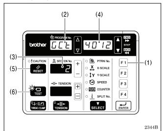
Once the grease has been applied, follow the procedure below to reset the cumulative number of stitches between grease applications.
