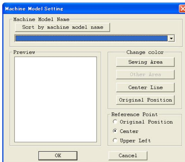
2. Select **B434E** from the **Machine Model Name** drop-down list.
