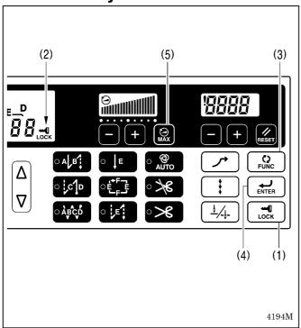
When the power switch is turned on, the LOCK key (1) turns ON. (The icon (2) is illuminated.)
