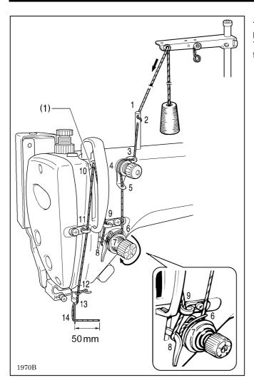
Turn the machine pulley and raise the thread take-up (1) before threading the upper thread.
