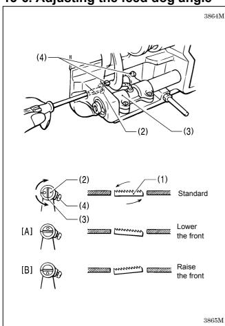
The standard angle for the feed dog (1) when it is at its highest position above the needle plate is when the " $\bigcirc$ " mark on the shaft (2) is aligned with the feed rocker bracket arm (3) and the feed dog (1) is parallel to the needle plate.
