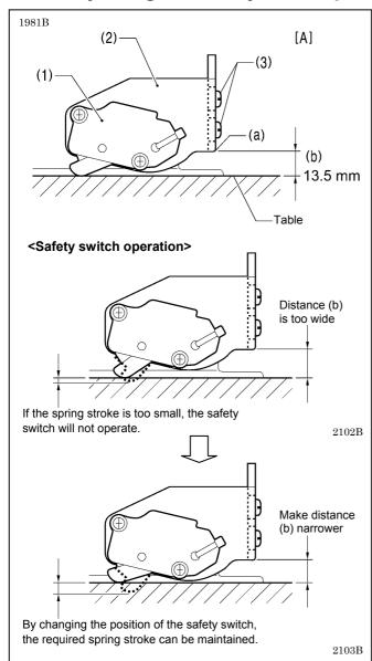
The standard position for the safety switch (1) is when the distance (b) between part (a) of the safety switch plate (2) and the table is set to 13.5 mm as shown in Figure [A]. If the processing method for the table results in distance (b) being too wide, it may adversely affect the operation of the
