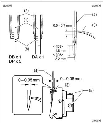
The tip of the rotary hook (3) should be aligned with the center of the needle (4) when the needle bar (1) moves up from its lowest position to the position where reference line (b), which is the line at the bottom of the needle bar (1) (third line from the bottom when using a DA x 1 needle), is aligned with the lower edge of the needle bar bush D (2) as shown in the illustration.
