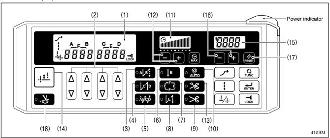
The power indicator illuminates when the power switch is turned on.
