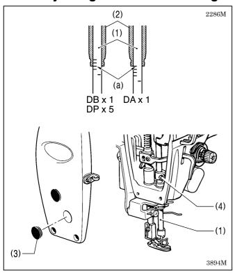
Reference line (a), which is the second line from the bottom of the needle bar (1) (fourth line from the bottom when using a DA x 1 needle) should be aligned with the lower edge of the needle bar bush D (2) as shown in the illustration when the needle bar (1) is at its lowest position.
