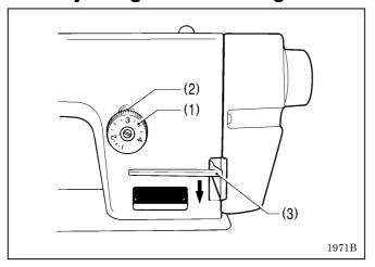
Turn the stitch length dial (1) until the desired stitch length number is aligned with the pin (2) above the dial.
