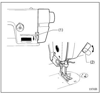
When the reverse lever (1) or the actuator switch (2) is pressed during sewing, the feed direction will be reversed. When it is released, the feed direction will return to normal.
