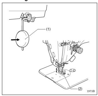
The presser foot (2) can be raised by pressing the knee lifter plate (1).
