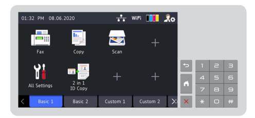
Remote Panel offers remote access to the front panel of the device through an Embedded Web Server (EWS). Enables remote configuration, as well as checking machine status, error conditions, and service reports. Helps reduce personal contact with the printer.
