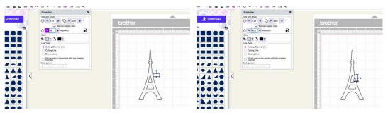
**step 11.** Move the tab so that two of the corners are overlapped with the side of the tower.
