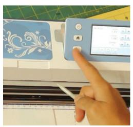
step 4. Make sure you install the deep cut blade (purple) for this project. You may also need to press the wrench button next to the screen to adjust your cut depth and cut speed settings. (I use Cut Speed: 1 and Cut Pressure: 5.) Play around on a scrap piece until you get it just right.
