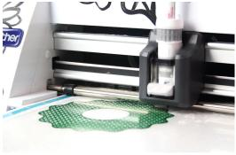
**step 7.** After the drawing is finished, remove the Universal Pen Holder and put a blade in place.
