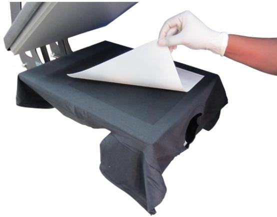
8. Press the garment using a hot press at 356°F for 35 seconds with 80psi to dry (cure) the pretreat. Cover the pretreated area with a Teflon sheet or use a Teflon cover (bra) on the upper heat element and lower platen base. This will give you the best results for both pretreat and ink curing.
