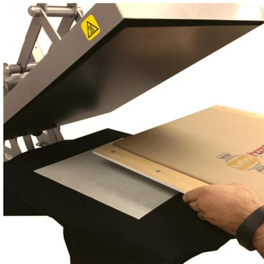
7. Press the garment using the Pretreat Paper Platen on the hot press for 35 seconds at 60 to 65psi. This is a cold press and is designed to transfer over the pretreat solution from the paper with no heat. On this application the heat is not a factor as the Pretreat Platen pad obstructs the heating element.
