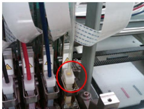
16. Place the cable (silver side up) into the black tabs from step 10, and lock into place by pushing the tab away from you (towards the capacitor).
