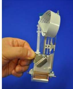
12. Mount the print head on the printer; fit the V-shaped groove to the positioning pin.
