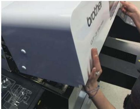
8. The example being shown is for the color print heads, when installing the white print heads, prepare maintenance solution, maintenance cartridge, and follow the prompts on the screen.
