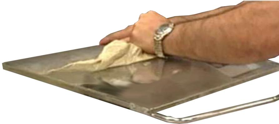
4. After removal of the old platen sheet clean the surfaces of the Platen using a soft cloth dampened with mild detergent, and then wipe it dry using a soft and dry cloth.
