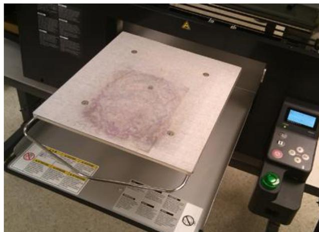
2. Use a cleaner that is conducive to removing the adhesive from the platen. “Goof Off” or a similar product will work fine. It is recommended to test prior to using any cleaning solvent so you don’t damage the platen material.
