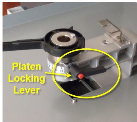
2. Remove the Black platen height adjustment lever by removing the silver screw that blocks the lever from being removed. Thread the screw back into place for safe keeping.
