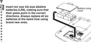
Attach the battery compartment cover by inserting the three hooks at the bottom into the slots on the machine, then pushing down firmly on the cover until it snaps into place.
