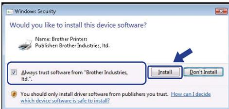
**9** When this screen appears, connect the USB interface cable to your PC, and then connect it to the machine.
