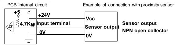
• Insulate input using a relay if not using a contact switch or a 24 V sensor.
