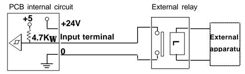
• Use a relay for electronic circuit whose maximum applicable load is 5 V and 1m A or less.
