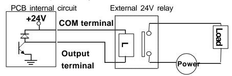
• No fuses are built in the output circuit. To prevent circuit damage when forming short output, it is recommendable to install an external fuse on each output.
