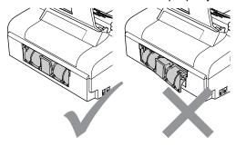
6 Open the Upper Jam Clear Cover (1). Make sure that there is no jammed paper left in the corners of the machine.
