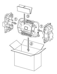
9 Pack the printed materials and additional parts in the original carton as shown below. Do NOT pack the used ink cartridges in the carton.
