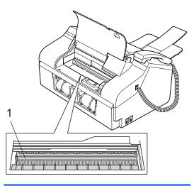
Clean the machine printer platen (1).
