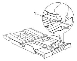
3 Press and slide the paper side guides (1) and paper length guide (2) to fit the paper size.
