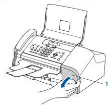
Pull all the lock release levers down and remove the yellow protective part (1).
