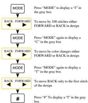
To move the frame in small increments
