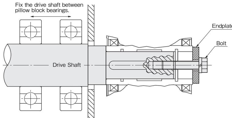
**Figure-3: Attachment Using an Endplate**
