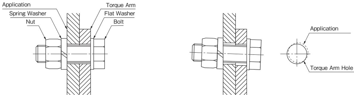
Figure 6: Fastening the Detent
