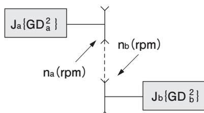
The inertia moment J<sub>b</sub> (GD<sub>b</sub><sup>2</sup>) of the load can be converted into the equivalent value at the n<sub>a</sub> shaft as shown below:
