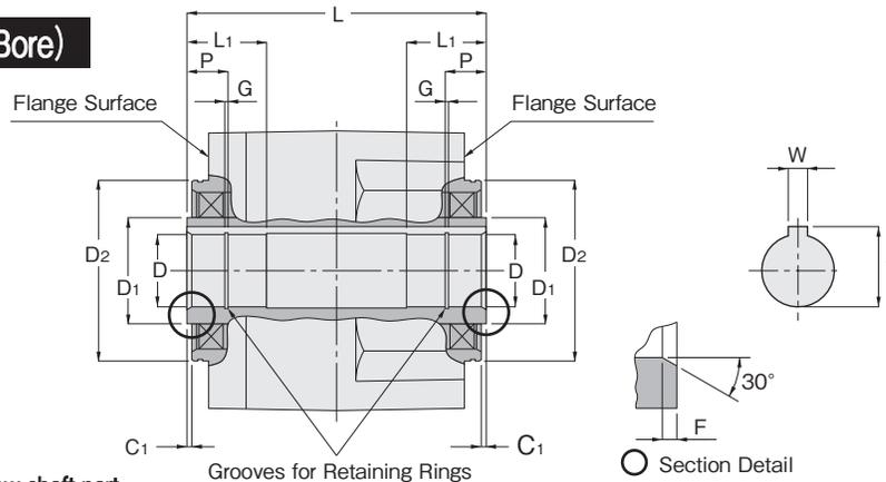
Detailed dimension table for the hollow shaft part
