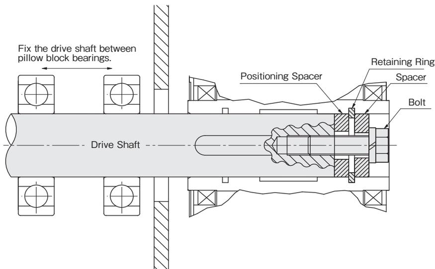
**Figure-4: Attachment Using a Space and Retaining Ring**
