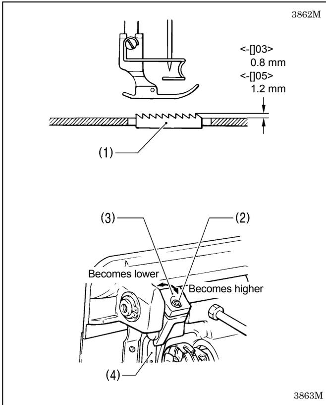
The standard height of the feed dog (1) when it is at its maximum height above the top of the needle plate is 0.8 mm for -□03 specifications, and 1.2 mm for -□05 specifications.
