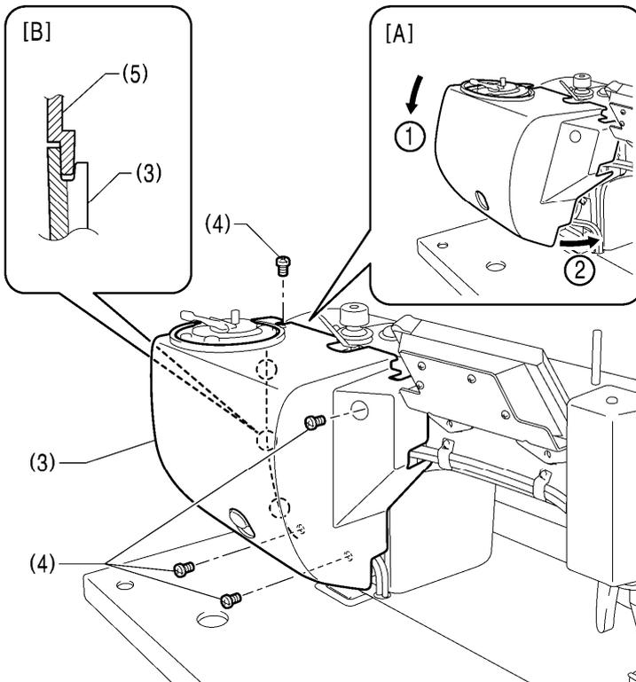
2. Install the motor cover (3) as shown in Figure [A], and then securely tighten it with the four screws (4).
