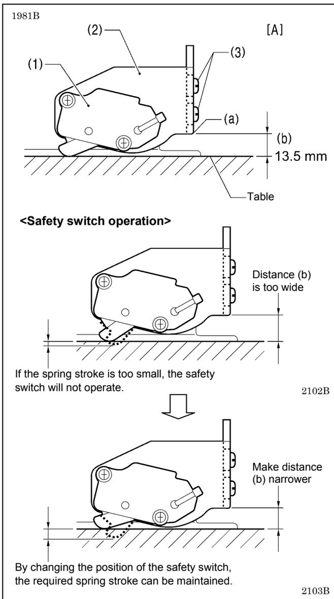
The standard position for the safety switch (1) is when the distance (b) between part (a) of the safety switch plate (2) and the table is set to 13.5 mm as shown in Figure [A]. If the processing method for the table results in distance (b) being too wide, it may adversely affect the operation of the safety switch (1).
