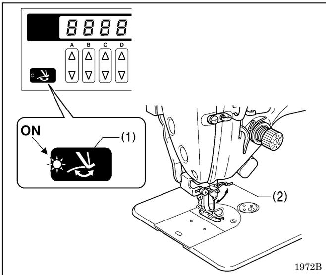
Press the thread wiper key (1) on the operation panel so that the indicator illuminates. If this is done, the thread wiper (2) will operate after the thread is trimmed.
