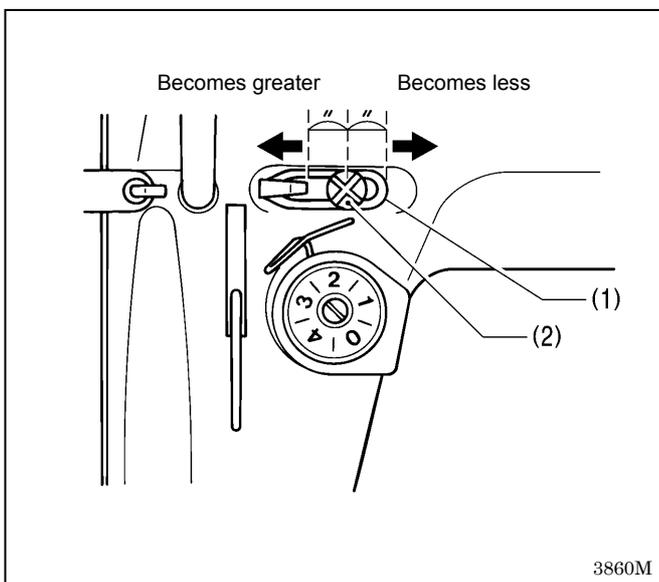
The standard position of arm thread guide R (1) is the position where the screw (2) is in the center of the adjustable range for arm thread guide R (1).
