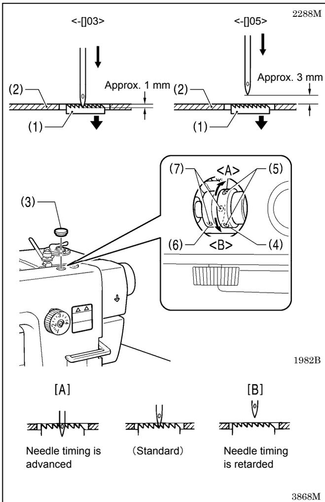
The illustration at left shows the standard position for the needle tip when the feed dog (1) is lowered from its highest position until it is flush with the top of the needle plate (2).
