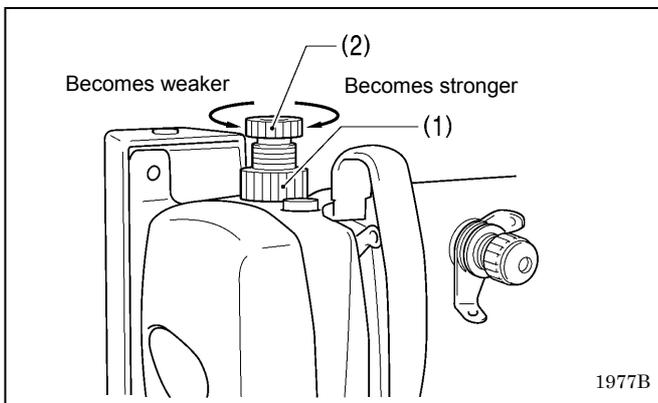
The presser foot pressure should be as weak as possible, but strong enough so that the material does not slip.
