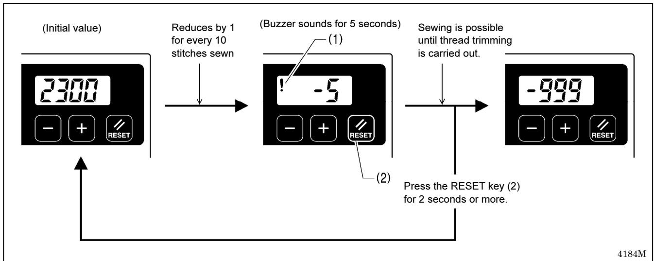
1. When sewing is carried out, the value shown in the lower thread counter display is reduced by 1 for every 10 stitches sewn. (When the value goes below zero ("0"), a minus sign appears and counting continues to a maximum of "-999".)
