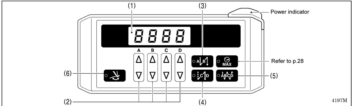
The power indicator illuminates when the power switch is turned on.
