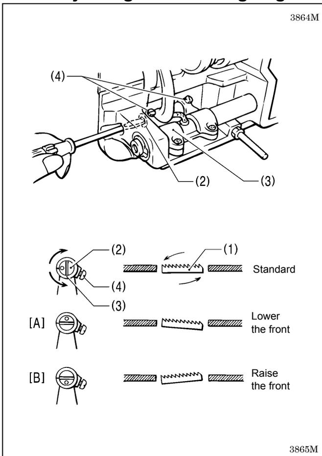
The standard angle for the feed dog (1) when it is at its highest position above the needle plate is when the “O” mark on the shaft (2) is aligned with the feed rocker bracket arm (3) and the feed dog (1) is parallel to the needle plate.
