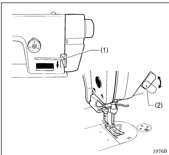
When the reverse lever (1) or the actuator switch (2) is pressed during sewing, the feed direction will be reversed. When it is released, the feed direction will return to normal.
