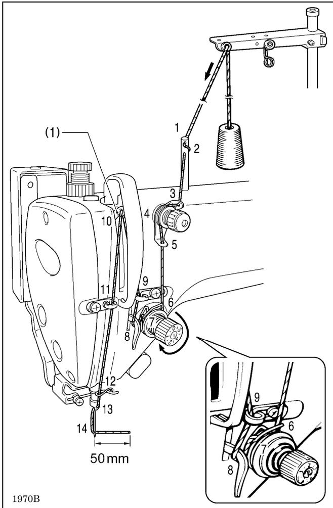
Turn the machine pulley and raise the thread take-up (1) before threading the upper thread. This will make threading easier and it will prevent the thread from coming out at the sewing start.
