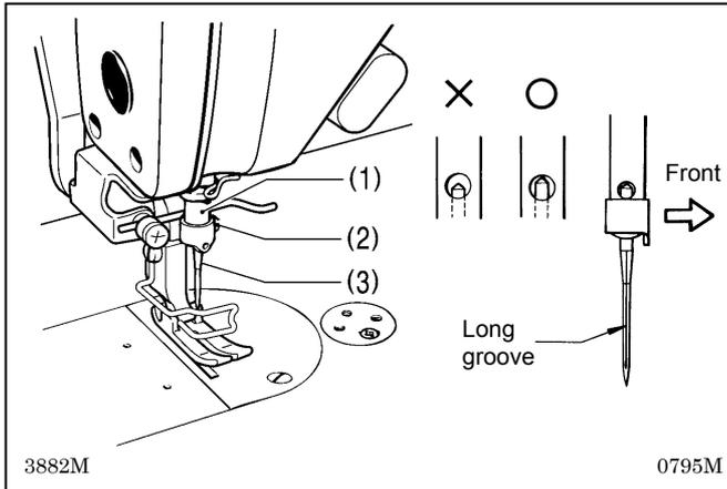
1. Turn the machine pulley to move the needle bar (1) to its highest position.
