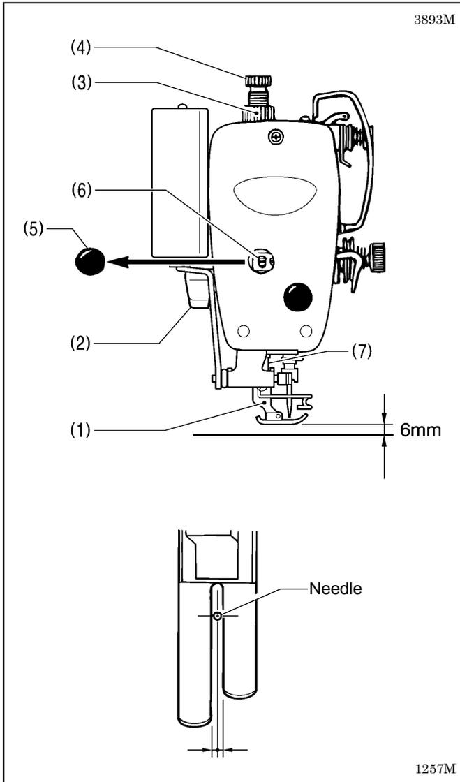
The standard height of the presser foot (1) is 6 mm when the presser foot (1) is raised by means of the lifting lever (2).
